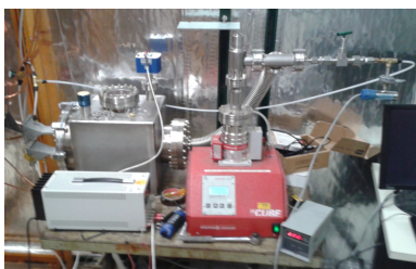
Figure 13: Setup at MTest in the gas room. the module is placed inside the vacuum tank and pumped down using the Pfeiffer turbo vacuum pump. The gas is supplied from MTest.
