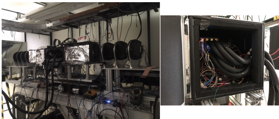
Figure 23: A picture of the experimental area. The pixel telescope detectors are placed inside the electrostatic-discharge shielded boxes on the two sides of the DUT area. Cold box with mounting frames for LGAD sensors is shown on the right.
