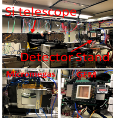
Figure 26: Detector setup in beamline, including use of FTBF Si telescope.
