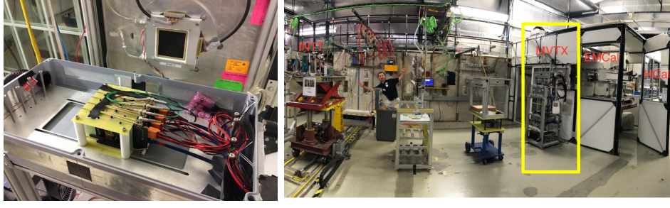
Figure 30: (Left) The telescope box, with cover removed. Beam direction is from lower left to upper right. (Right) sPHENIX detectors in the MT6.2 area, beam is left to right.
