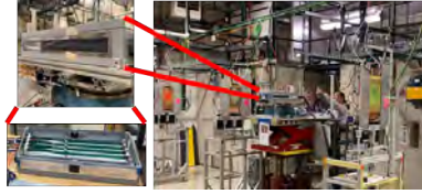
Figure 35: MVTX Telescope Setup at FTBF. A 4-stave telescope assembly was used at Fermilab to verify the detector tracking performance with the latest near final readout electronics and high-speed data cables, and production sensor staves.
